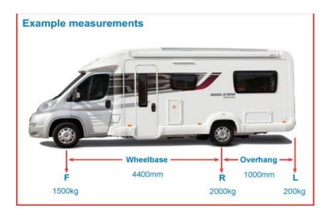
To work out the effect this will have on the motorhome's front and rear axle loads we can use the formula, and simply replace the letters with the values in the example diagram above.
